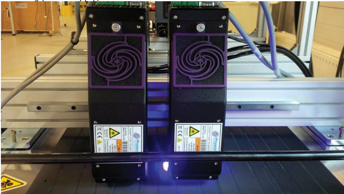
2 x LED Curing lamps of 75 mm curing width each.
