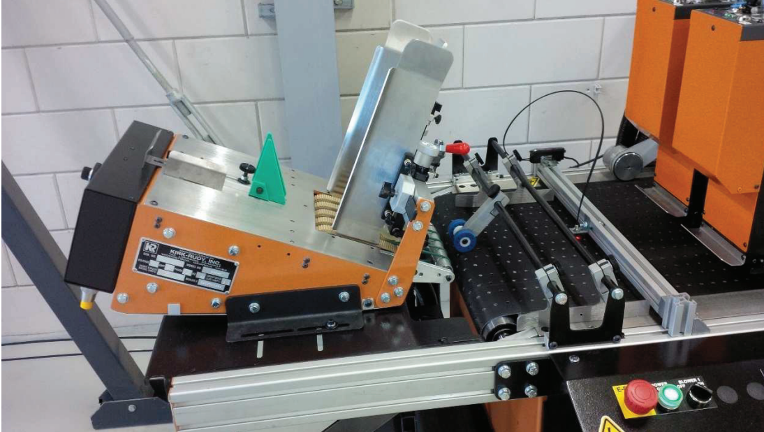
KR496F Product Specifications: Up to 355 mm wide and 300 mm long. With single roller kit for narrow product of minimum 35 mm wide.
